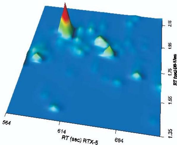
Figure 4: A zoomed-in view of the area in the box in Figure 3 showing greatly increased detectability offered by GCxGC.
