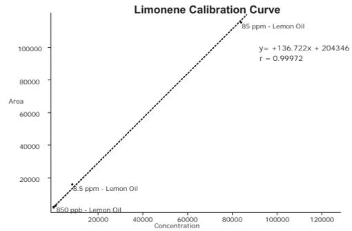
Figure 5: The calibration curve for limonene with concentrations from 8.5 ppb to 85 ppm.
