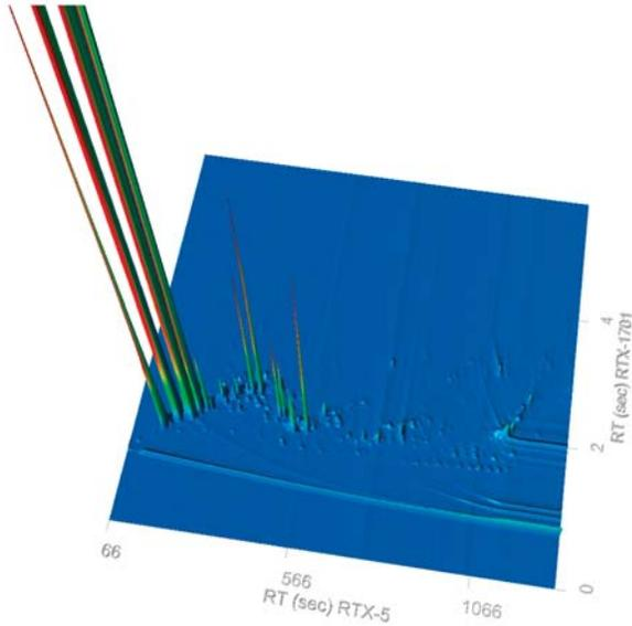
Figure 3: An optimized GCxGC 3D plot of 1  $\mu\text{L}$  of lemon oil at a split ratio of 300:1. The Z-axis is scaled to show trace compounds.
