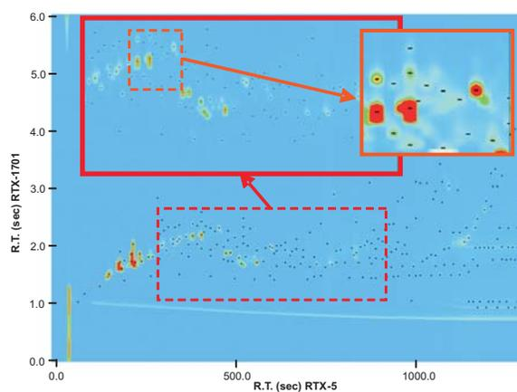
Figure 2: An optimized GCxGC contour plot of 1  $\mu$ L of lemon oil at a split ratio of 300:1. The inset is a magnification of an area which highlights the enhanced separation in the second dimension.
